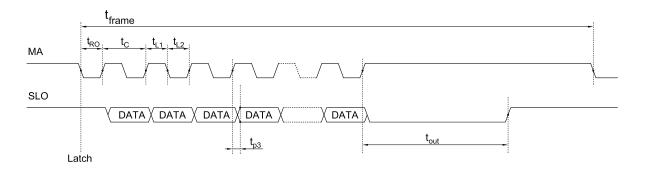
Figure 5: SSI Timing
