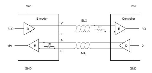
Figure 1: Point-to-point configuration
