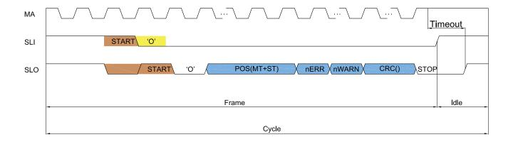
Figure 4: BiSS Frame Structure
