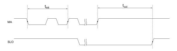
Figure 3: BiSS-C (SSI) Slave Timeout Sequence
