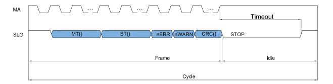
Figure 6: SSI Frame Structure
