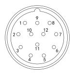
M23 12pin male socket pin distribution diagram
