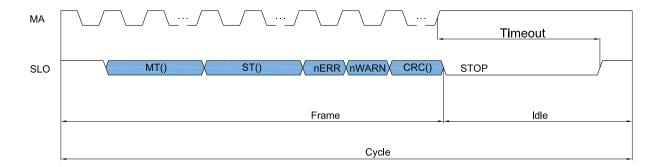
Figure 6: SSI Frame Structure
