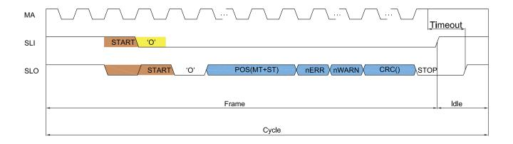
Figure 4: BiSS Frame Structure
