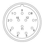
M23 12pin male socket pin distribution diagram
