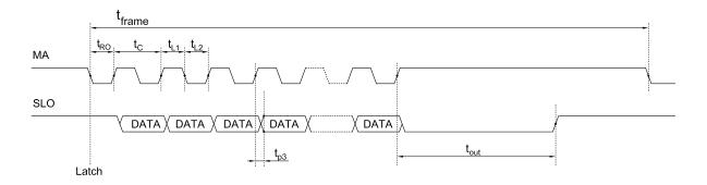
Figure 5: SSI Timing
