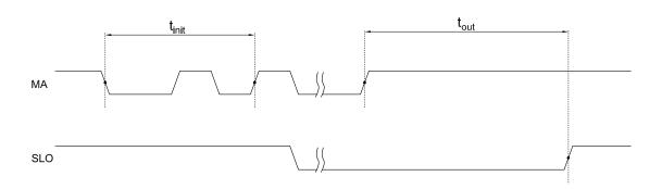
Figure 3: BiSS-C (SSI) Slave Timeout Sequence
