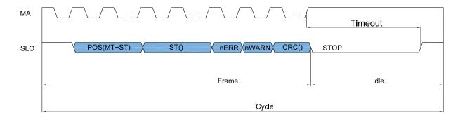
Figure 6: SSI Frame Structure
