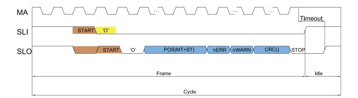
Figure 4: BiSS Frame Structure
