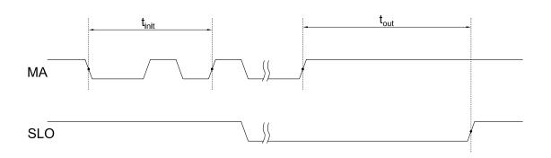
Figure 3: BiSS-C (SSI) Slave Timeout Sequence
