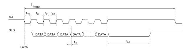
Figure 5: SSI Timing
